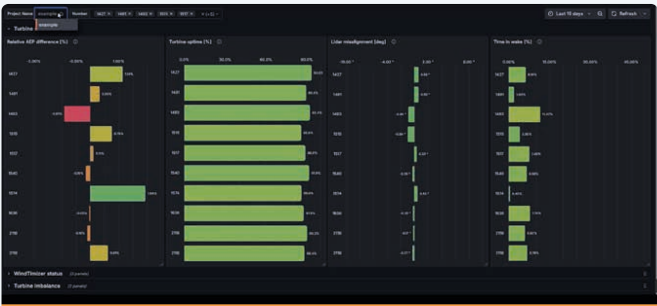
Overview of the performance of each unit in an entire wind farm equipped with the TPM-module
